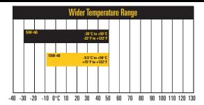
While Cat DEO SYN 5W-40 has the same high-temperature range as most SAE 15W-40 oils, its unique synthetic polyalpaolefin (PAO) molecular structure and higher viscosity index provide a better protective film at high temperatures. It also remains fluid at subzero temperatures and provides rapid cold-engine start-ups at ambient temperatures down to  $-30^{\circ}$ C ( $-22^{\circ}$ F).
