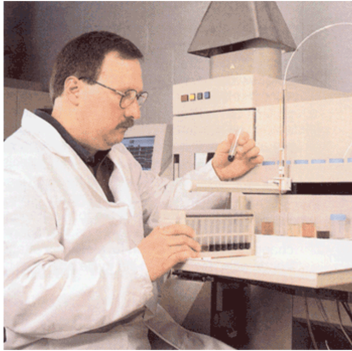
Analyzing an oil sample using an inductively coupled plasma spectrophotometer.
