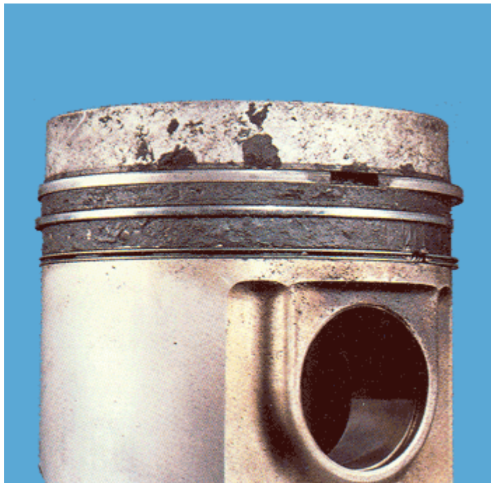
The heavy first and second land deposits indicate the oil can no longer keep the piston clean. The extreme degradation and deterioration of the oil maybe due to extended oil change intervals or improper oil performance classification selection.
