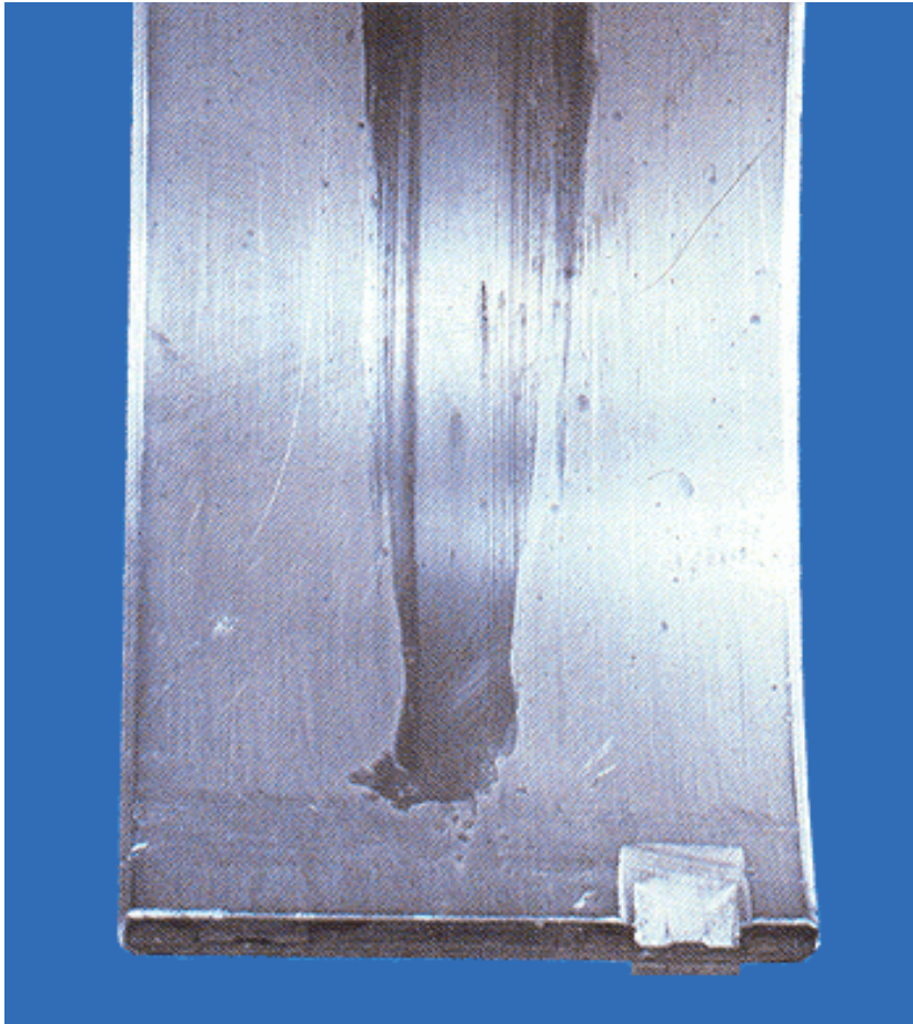
Bearing shows smearing, which is the initial stage of damage caused by lack of lubrication.
