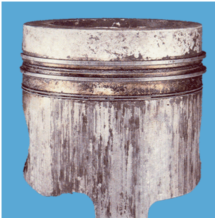
Seizure marks from top to bottom can indicate a cooling or lubrication system failure.
