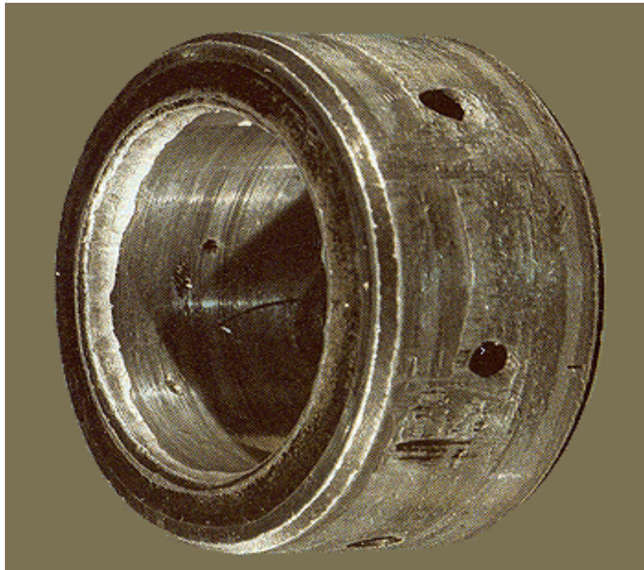
Oil holes damaged on the O.D. and reduced in size on the I.D. of journal bearing due to lack of lubricant.
