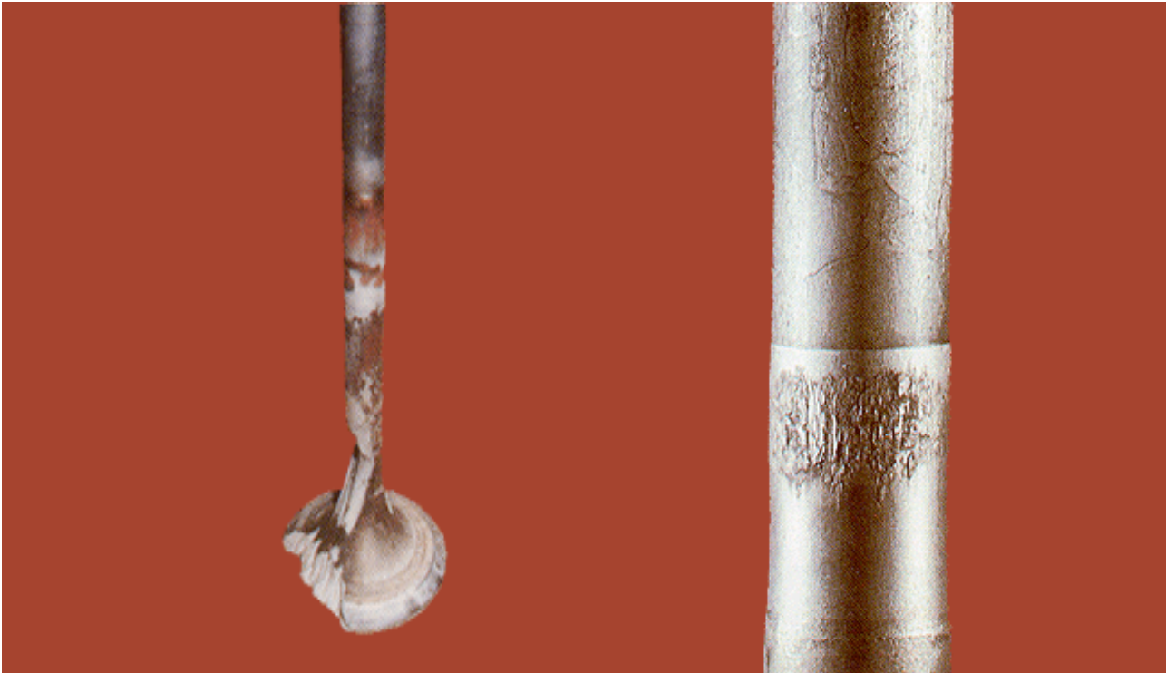
Valve guttering effect caused by excessive deposit formation.
