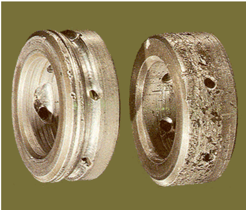
Deep scratches and damage to oil holes on bearings.
