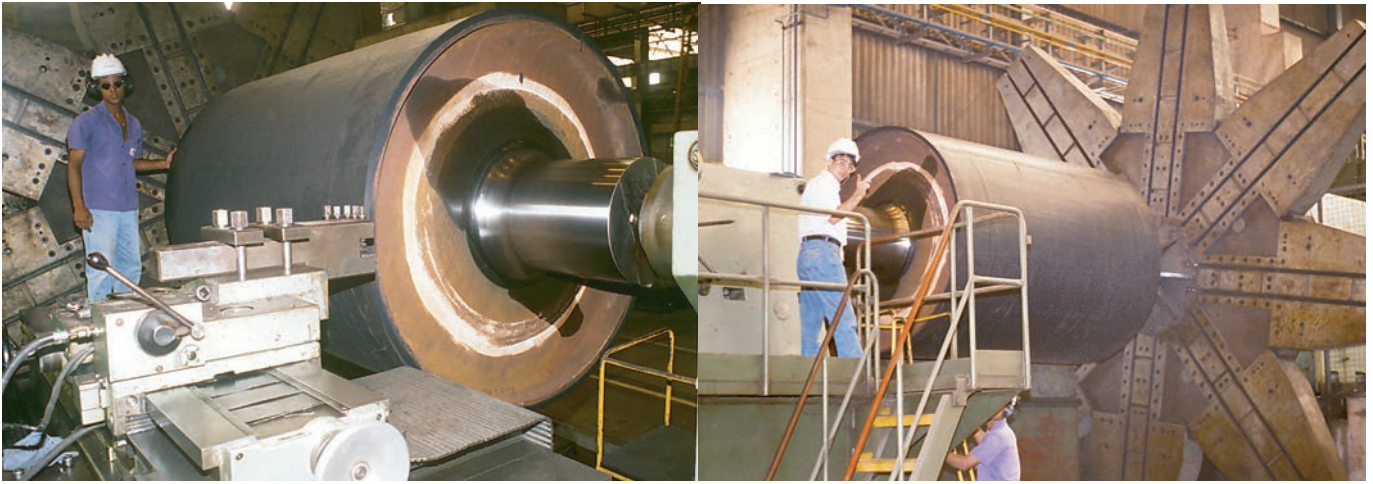
Shaftless pulley for heavy-duty application in installation.
