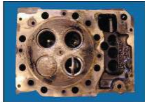
Figure 6 Add Charge Upper end failure – damaged cylinder head
