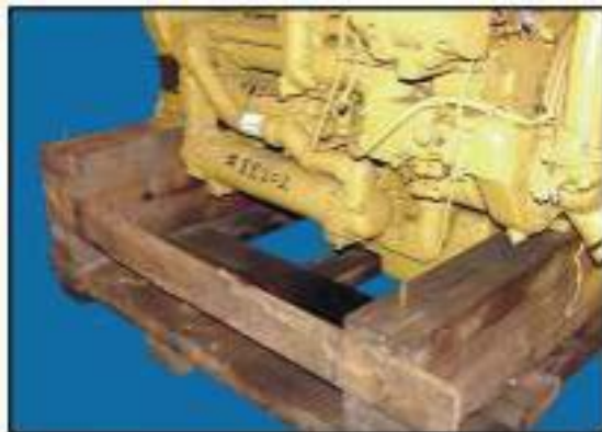
Figure 5 Add Charge Core not returned on correct stand
