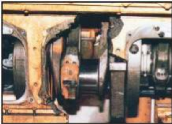
Figure 3 Damaged Core Refund Broken engine block
